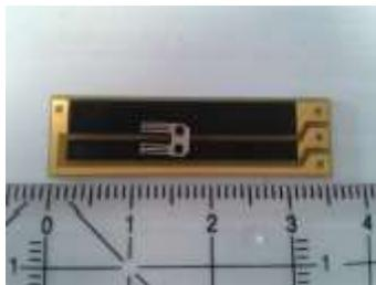
*CAPTION: Samples of the newest generation of conductive polymers used in H+K's ultra-thin Sensolnk potentiometer solution now offer two new additional features. They are self-lubricating which means that no grease has to be applied between the wiper and the polymer track. Because of the polymer's lotus effect, the new HK membrane potentiometers are now also water-repellent which opens a wide range of new applications.*
