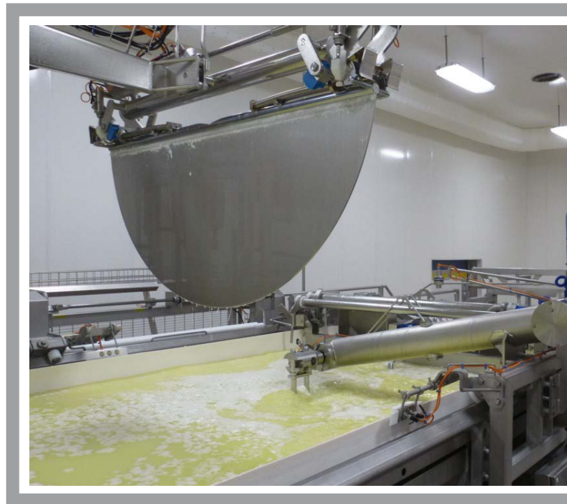
Image: A sophisticated partitioning system in the coagulator ensures safe processing according to the FIFO principle (first in- first out)
